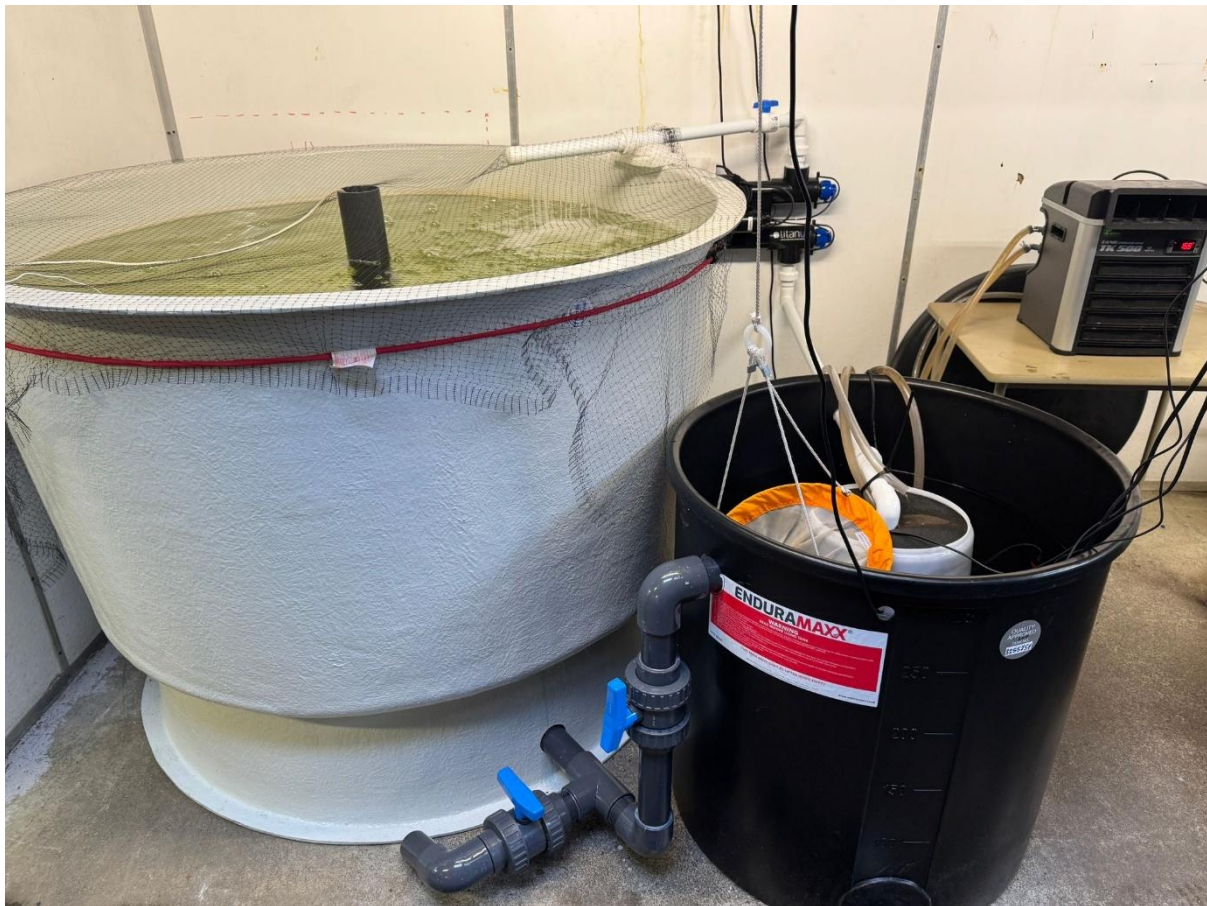
Figure 2. The recirculating propagation system in situ at the FBA's Species Recovery Centre.
